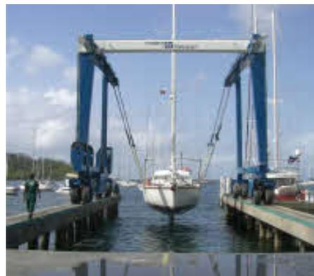
any essential under water bits and the boat was raised into the air. (We were no longer aboard.)The travel-lift, for such is the machine's name, rolled forward on its massive wheels and held the boat steady above the ground. A man with a jet hose scooshed water all over the hull for ever and a day.
