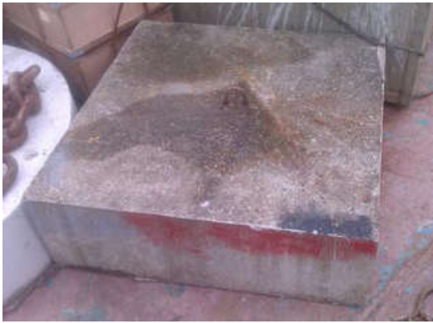
Figure 4.4 - Concrete Slab Sinker
